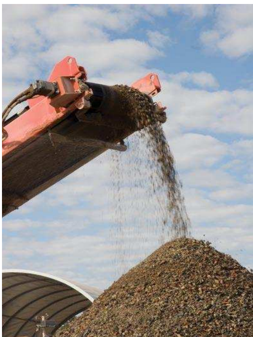
Developing markets and converting "waste" materials into useful end products. In addition to waste generated on individual construction sites, materials from the broader earthworks and civil works undertaken on a residential development can also be recovered – for example, to produce course aggregate or road base. This reduces demand for "virgin" materials and associated environmental impacts/costs.
